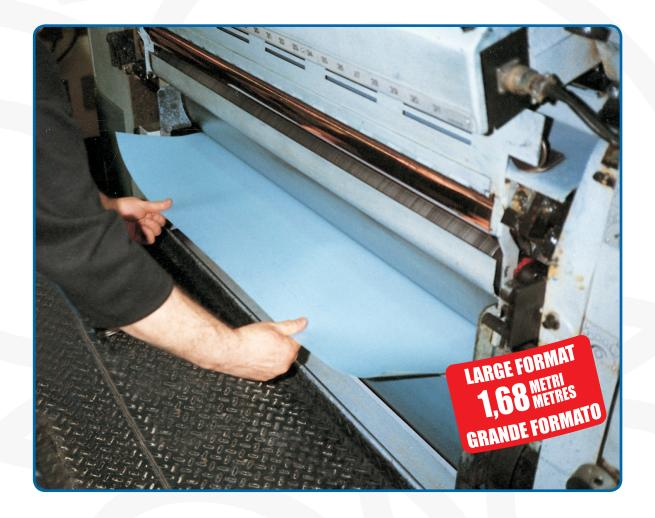
A range of calibrated underpacking polyesters that offer maximum dimensional stability, ensure the strongest adhesion and leave no residues after use
